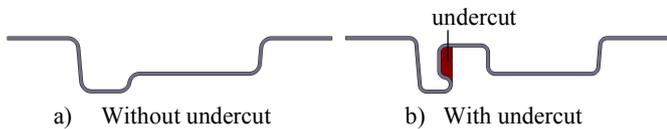
**Fig. 2** Sheet metal cross section
